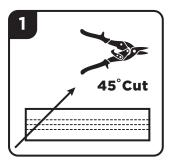
Using tin snips, cut out a 45 degree angled section of the downspout extension.
