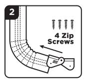
Slide the Zip Hinge onto the elbow of the down-spout and secure with zip screws. Make sure the Zip Hinge is fully seated before attaching.
