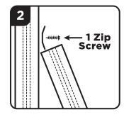
Use zip screw or 1/8" rivet to attach clasp 3/4 inches above raised extension.
