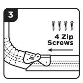
Slide the cut section of the downspout extension into the Zip Hinge and secure with zip screws. Make sure the down-spout is fully seated before attaching.
